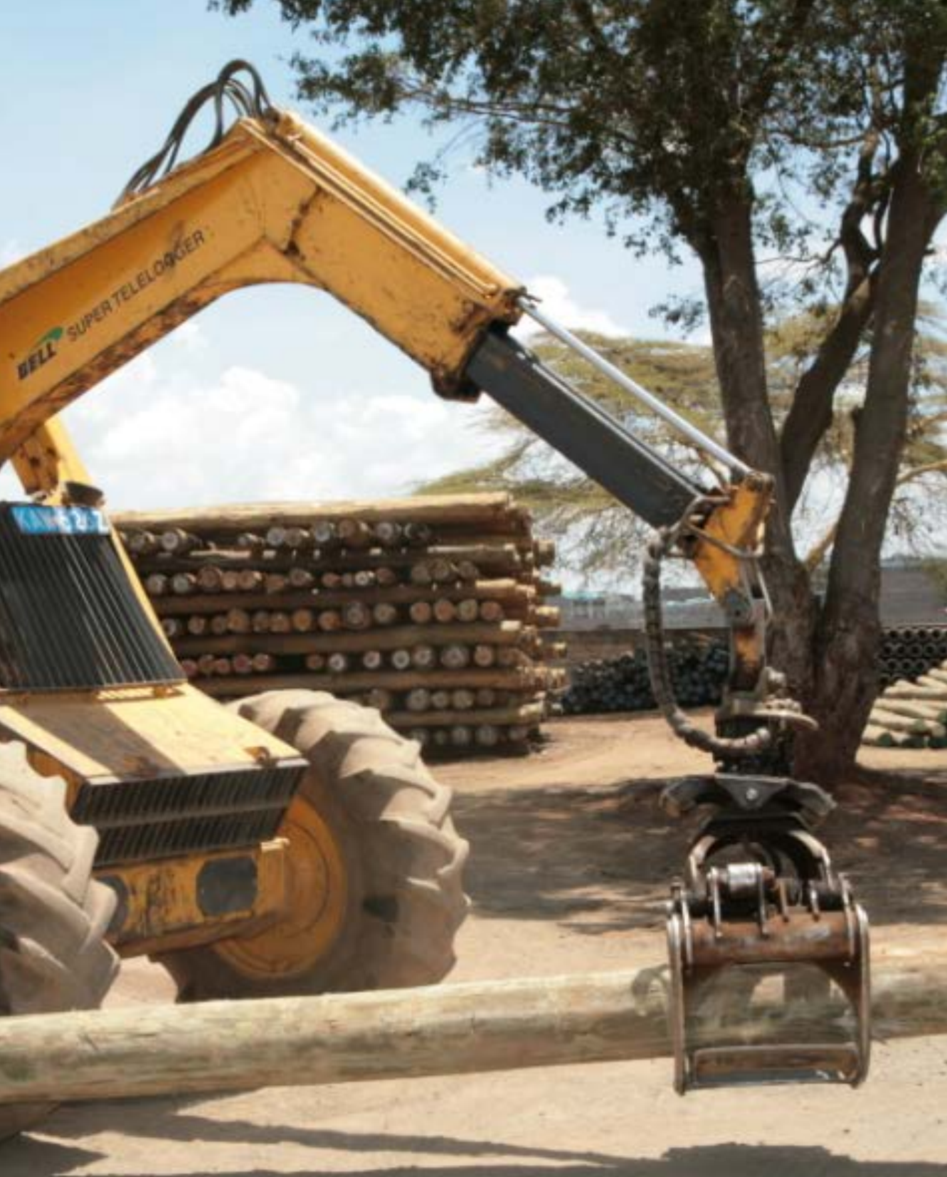
A telelogger machine, used to move and load poles
