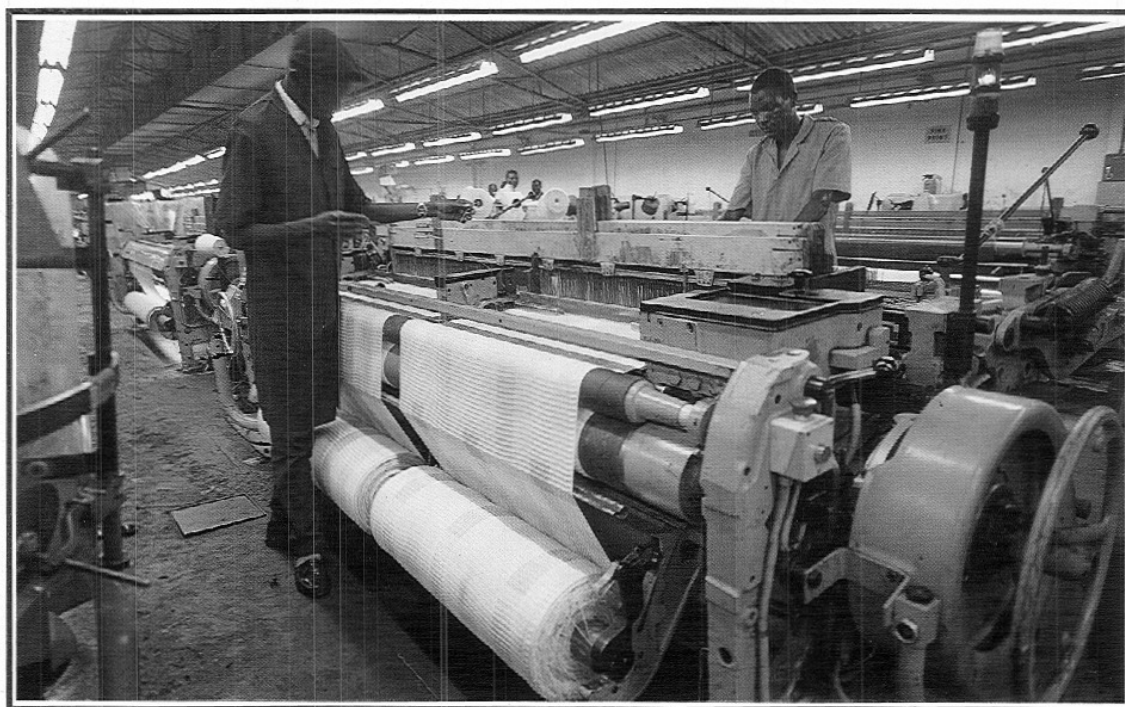
The Raymond Woolen Mills (Kenya) Limited an Associate Company of ICDC based in Eldoret, produces a wide range of fabrics. Picture above shows baby shawl material in production.
